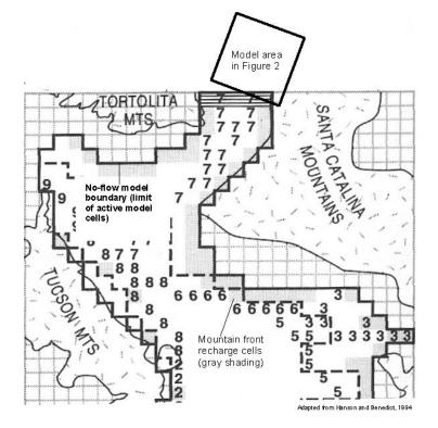
**Figure 1.** Model domain for northern part of Tucson Active Management Area model, showing  $1 \times 1$  mile cell size, mountain front recharge cells, and location of model shown in Figure 2.
