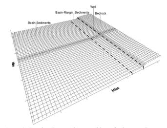
*Figure 3.* Simulated groundwater table in the basin sediments and bedrock aquifer system, with model grid superimposed (no vertical exaggeration).
