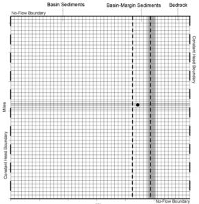
*Figure 2. Model grid, model boundary conditions, and hydrogeologic units (black dot shows well location).*
