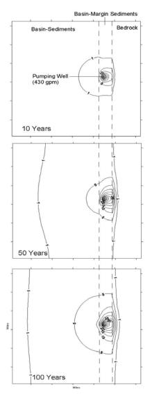
Figure 4. Simulated groundwater drawdown contours, in feet, from a single pumping well after 10, 50, and 100 years (dashed vertical lines show boundary of hydrogeological units).
